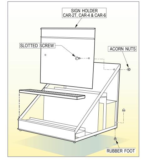
airpots. Place it against the back of the rack. Align the holes on the rack with the holes on the sign holder. Insert the slotted screws, (two provided) to fasten and secure with the acorn nuts.
